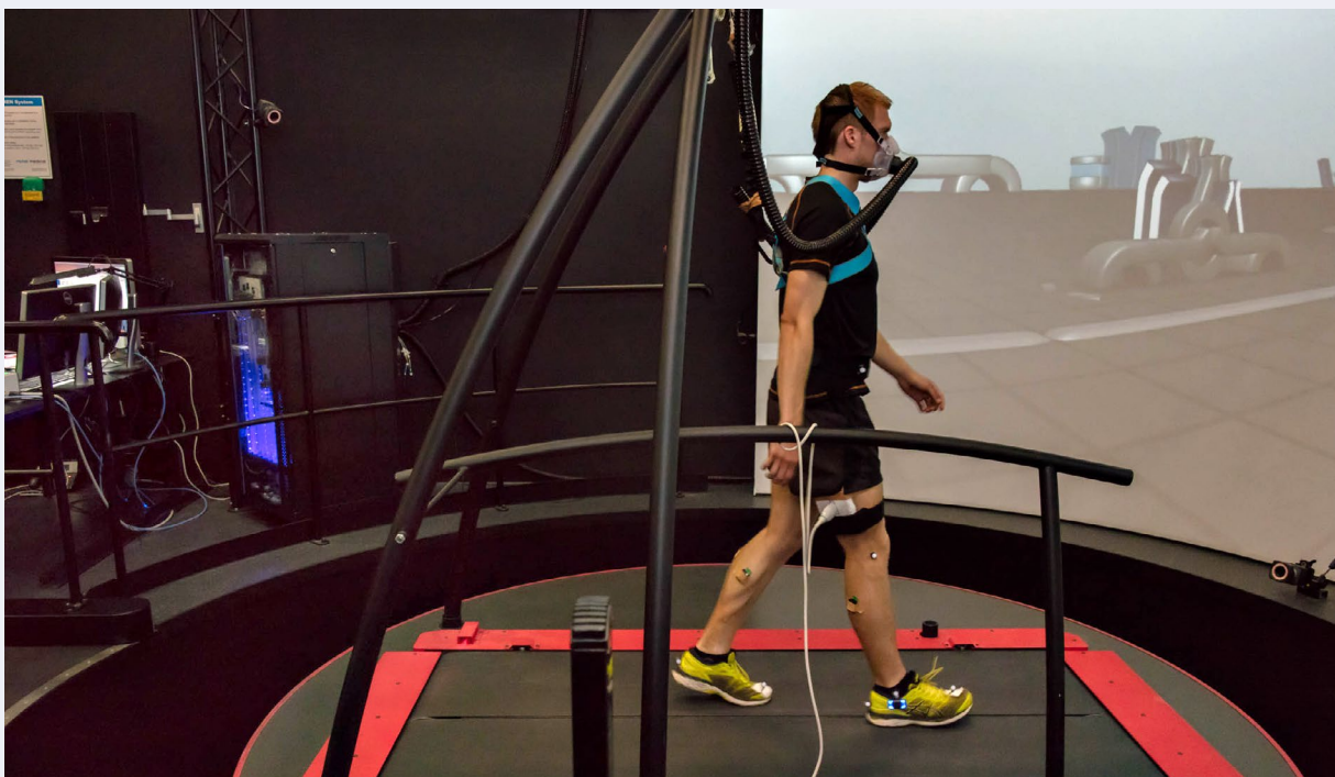
Figure 2 Snapshot of the CAREN system, one of the high-end facilities at the human performance lab. It includes a virtual environment, 3D motion capture, an instrumented treadmill and our in-house developed Omnicast setup for indirect calorimetry.
